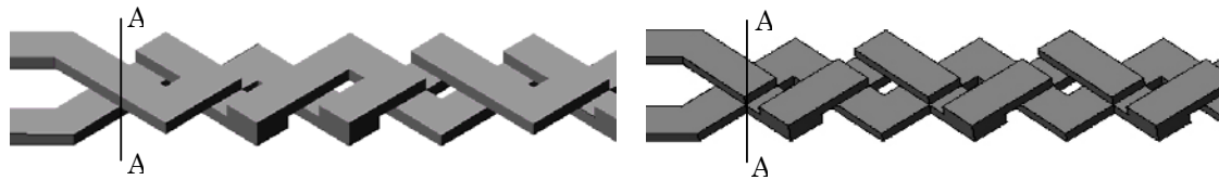
Fig. 1. Schematic of the chaotic mixer structure. Model A (left) and B (right).
